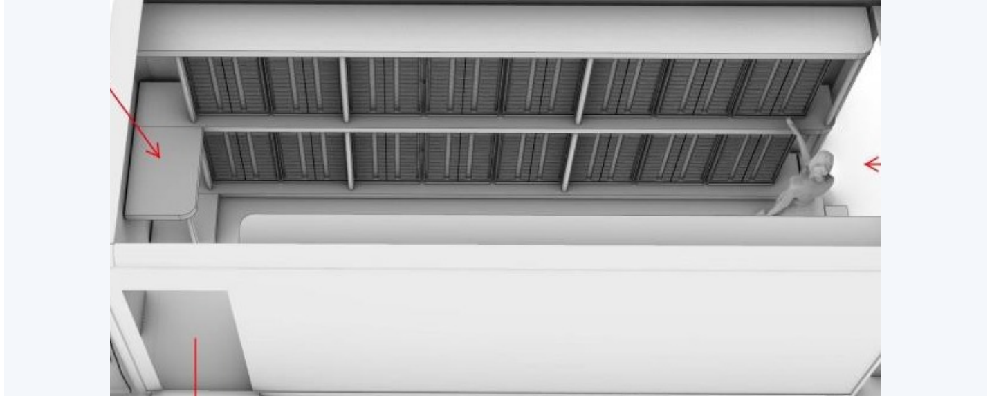
Cutaway view: 30 HL units on a racking system inside a 20–22 ft box truck. Entry at the rear, exit via built-in stairs to the cab.
